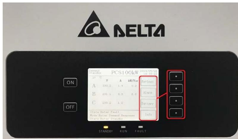
Figure 5. PCS Functional Keypad on Control Panel
