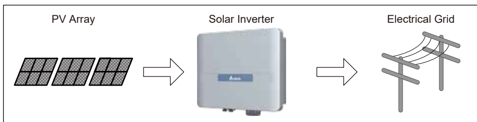
Figure 1-1 : Solar system operation illustration
