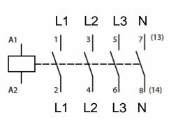
Pin A1, A2 = 24V aux. power cable Pin 1, 3, 5, 6 = AC input power cables Pin 2, 4, 6, 8 = output power cables connected to SMR
