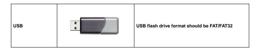
Put the firmware file provide by service team in the USB root path. Take update CHAdeMO CSU FW for example
