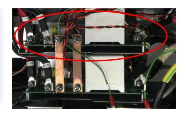
➤ Open front door and loose four screws
