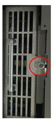
➤ Use screw driver to loose the screw
