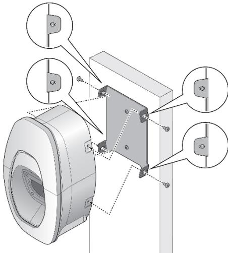
2. Align the EVSE with the screw holes on the mounting bracket.
