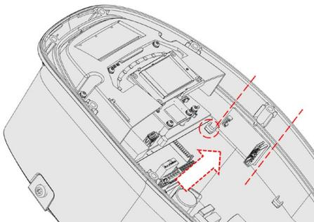
1. Based on the tenon, attach the connector to the inner surface of EVSE along the edge.
