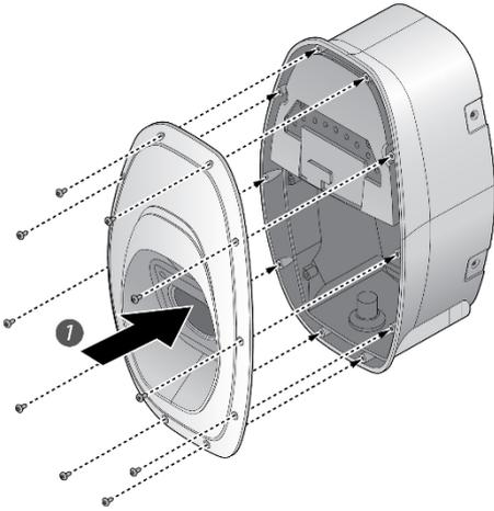
1. Recover the middle cover on the EVSE and secure the middle cover by using Torx T20 screwdriver.
