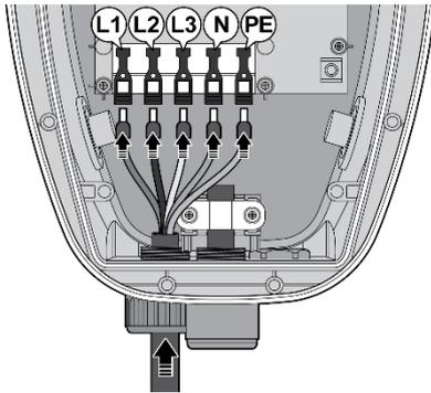
1. Install the copper wire as described. The section of copper wire connected to terminal shall be reserved enough tolerance to prevent any tension or stress from the external force.
