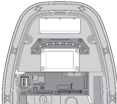
Configure the dip switches with following steps
