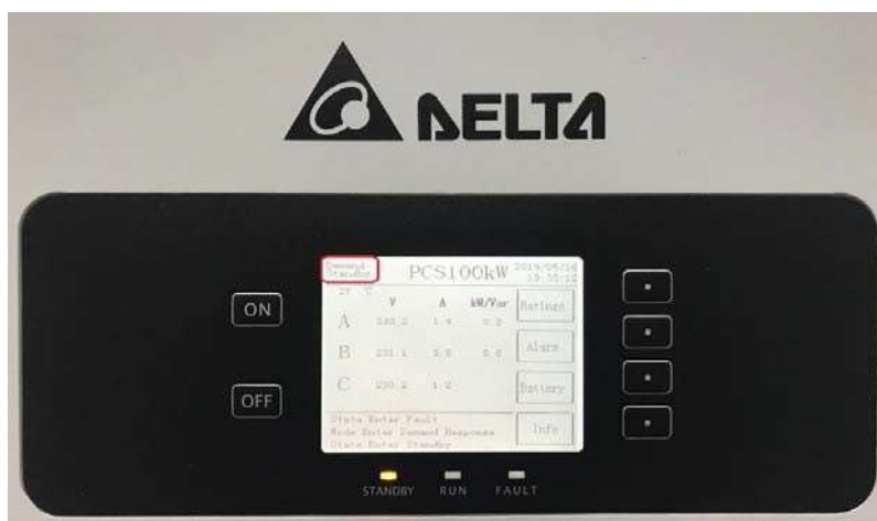
Figure 8. Operation Mode of PCS (2/2)
