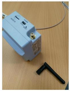
3. Screw the antenna extension to the DC1 antenna connection.
