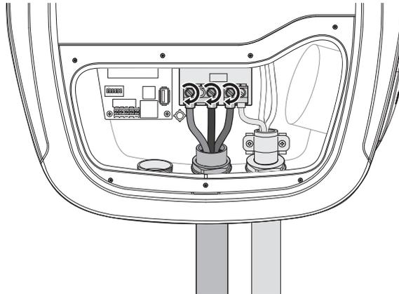
**Figure 10. Securing the Input Cable**
