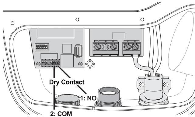
**Figure 13. Dry Contact Wiring Connection - WiFi Model**
