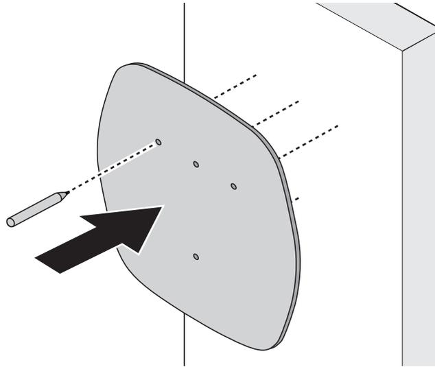
**Figure 3. Template for Marking the Screw Locations**
