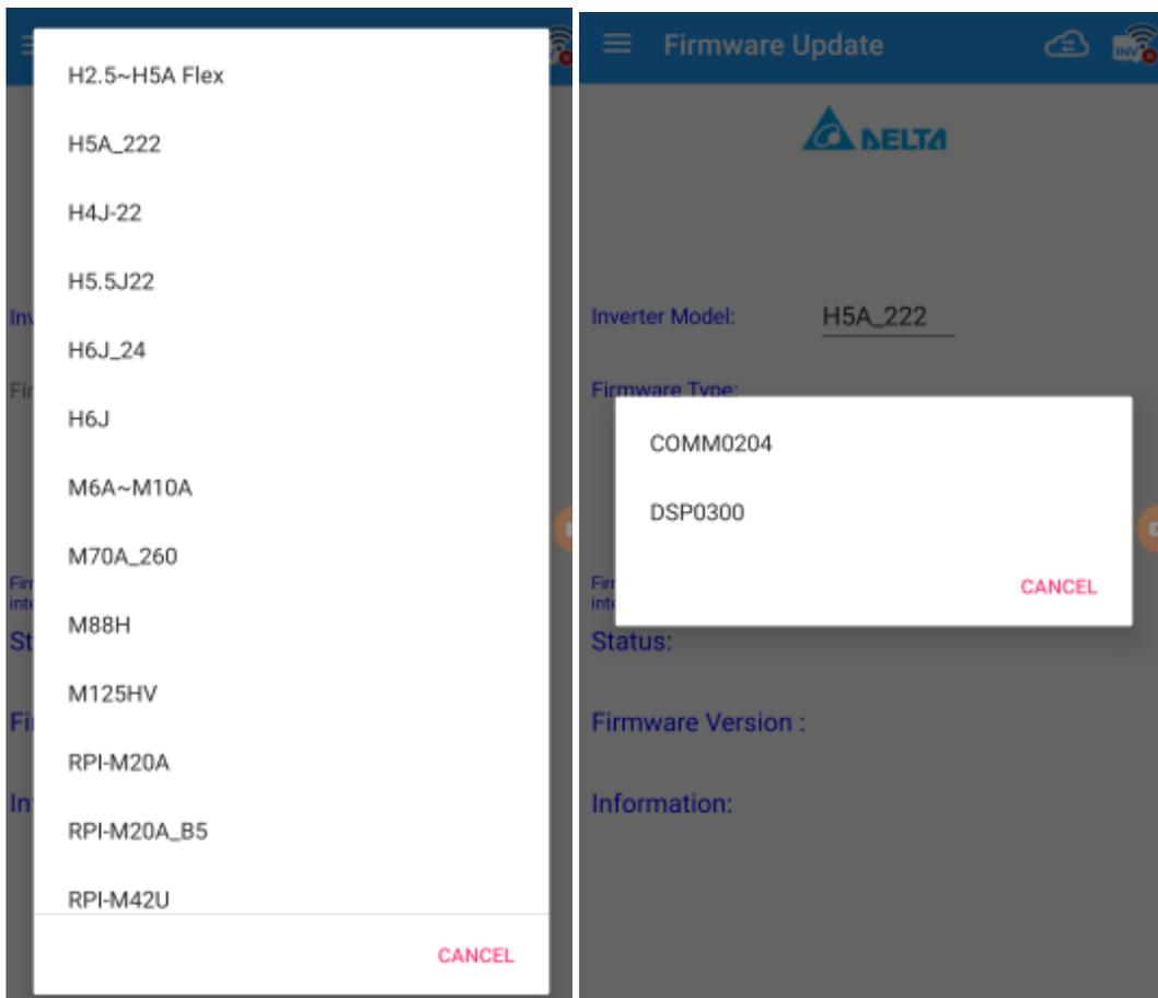
10. When Inverter Model and Firmware type has been selected tap “Load Hex File”
