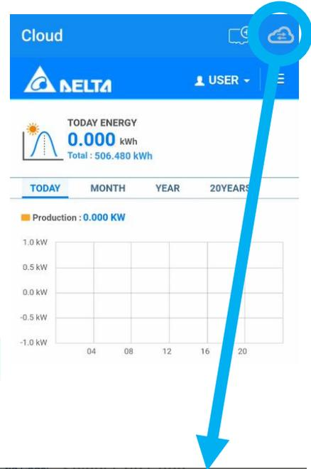
4. Press "OK" and your screen will swap to the Wi-Fi screen. Connect your mobile device to the Wi-Fi of the inverter using the password of the cloud account used to setup the device.
