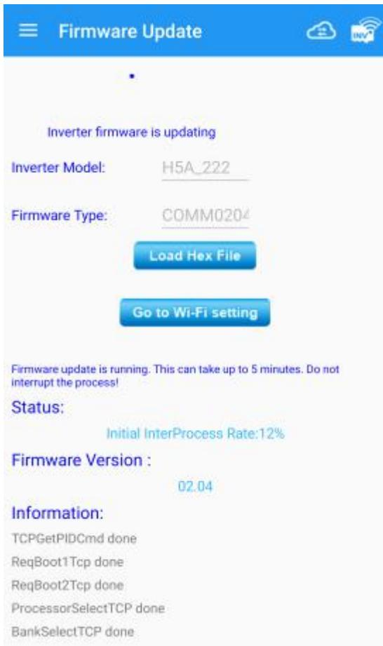
11. Press on the next button “Go to Wi-Fi setting” and connect your phone back to the inverter Wi-Fi. Then press Update Inverter.
