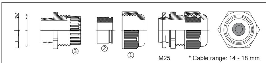
1. Loosen the front cover ① counterclockwise.
