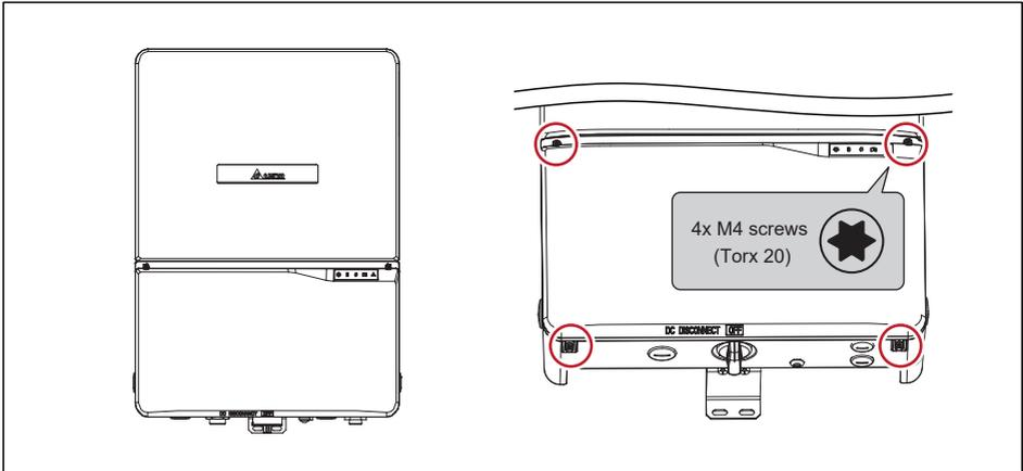
Figure 5-2 : Remove the wiring box cover
