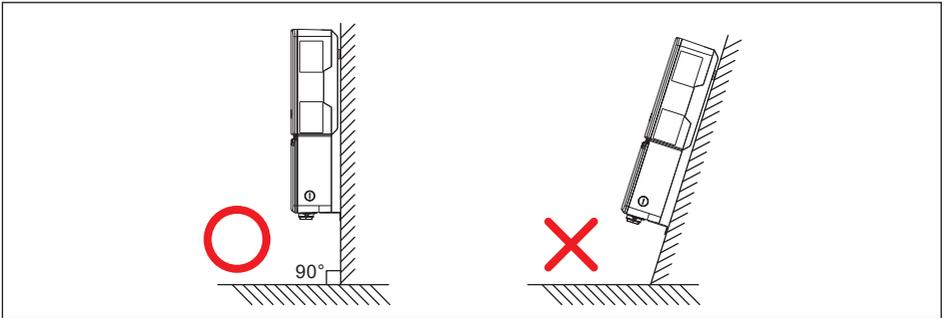
**Figure 4-2 : Correct and incorrect installation illustration**
