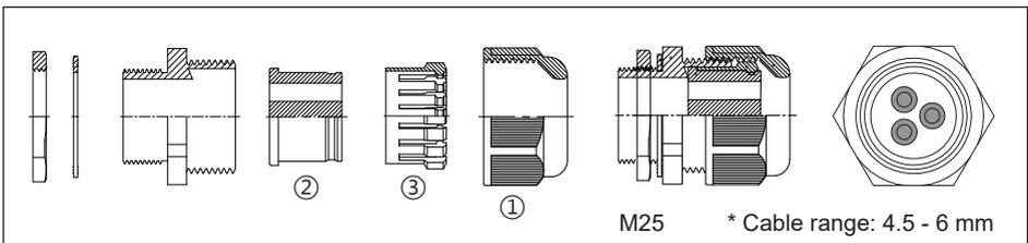
1. Loosen the front cover ① counterclockwise.
