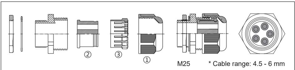
1. Loosen the front cover ① counterclockwise.
