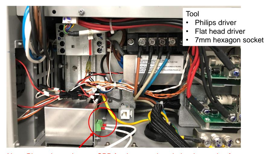
Note: Photo shows the new SPD for Japan region, below instruction focus on how to disassembly SPD and terminal.
