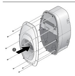
1. Recover the middle cover on the EVSE and secure the middle cover by using Torx T20 screwdriver.
