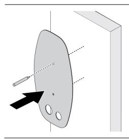
The EVSE is a stationary wall-mounted equipment. Using the template to mark the screw locations for the mounting bracket and cable holder (optional).
