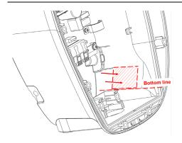
1. Based on the bottom line, attach the control board to the inner surface of EVSE.
