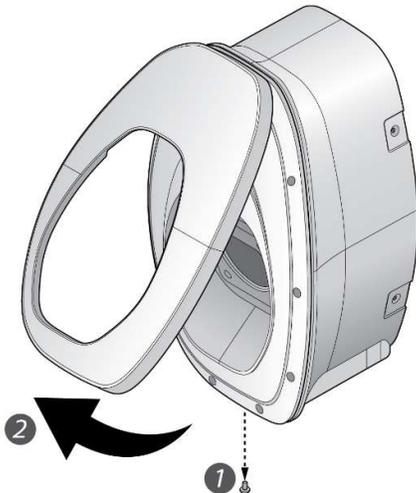
1. Remove the screw located at the bottom of front cover by using a Torx T20 screwdriver.
