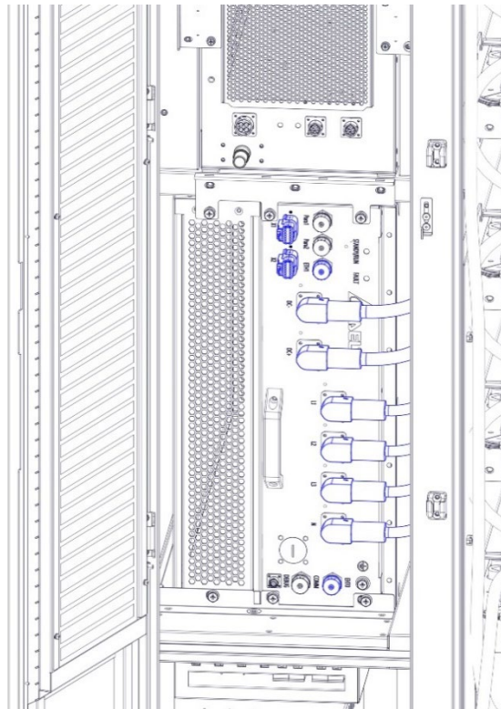
Figure 4-14 Re-connect power cable and signal wires
