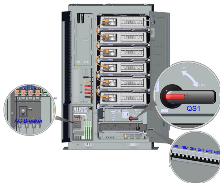
Figure 4-8 Turn off AC breaker & DC isolation switch and auxiliary power switch
